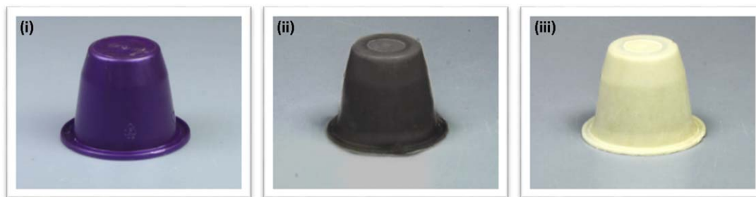
Figure 15. Coffee capsules: (i) polypropylene; (ii) PLA/GNP; and (iii) PLA/A-fSiO 2 . [Color figure can be viewed in the online issue, which is available at wileyonlinelibrary.com .]
